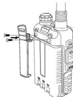
*Do not use any form of glue to fix the screws on the battery clip.*
