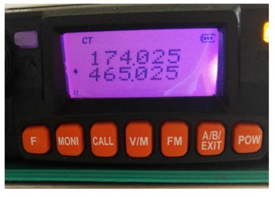
On the other radio select the upper display (with the A/B Button). Set the frequency to 136.025MHz (or your own VHF frequency)
