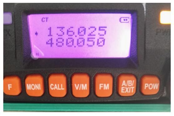
2: On <u>both</u> BTECH mobile radios set the PL Tones with MENUS 11 and 13. In this example set R-CTCS (Menu 11) to 74.4Hz and T-CTCS (Menu 13) to 74.4Hz
